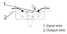
Connect the wires to the ceramic block as shown in the diagram below. Check the stability of the connection. For more safety in wires connection there should be used a metal sleeve to connect the two wires in the one terminal.
