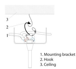
Attach the aluminum ties by connecting the steel wire with the wire, starting from the bottom of the installation box.
